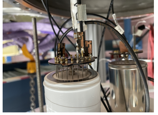
FIG. 4. Foreground: modified PMT base in experimental apparatus PATRIC. The left connection is the anode probe. The two right connections are the high voltage supplies. Background: unmodified control PMT.
